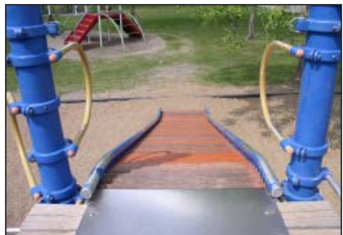
Roller slides should be inspected for pinch/crush points.
